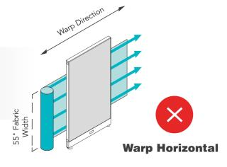
Fabrics cannot be applied warp vertical on panels with a width greater than 48 inches because panel width is greater than fabric width.
