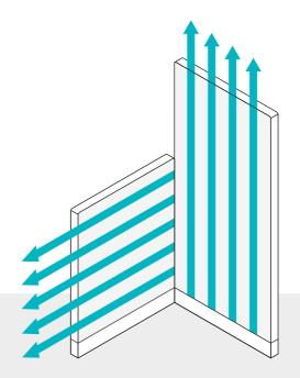
The combination of tall panels (height of 55 inches or more with warp vertical/off the roll) with short panels (height of 45 inches or less with warp horizontal) results in fabric patterns running in opposite directions.
